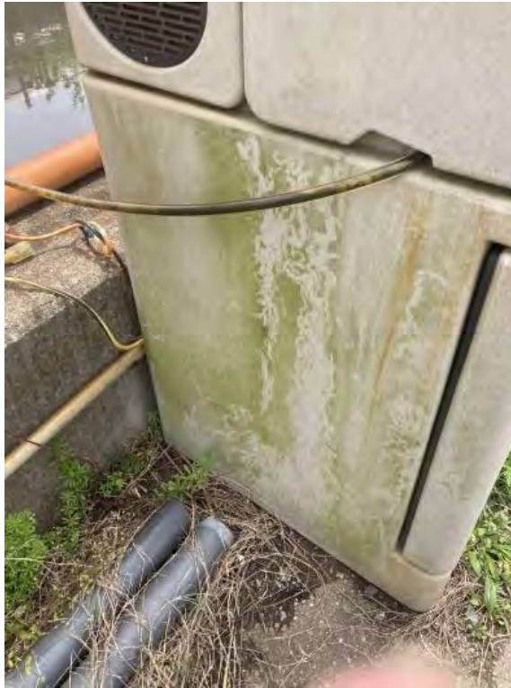
Figure 8 – Composite Autosampler Collecting NPDES Samples
