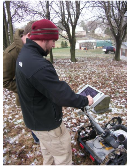
Above left: Tolson's Chapel from High Street. Above right: Jonathan Nichols of GEL Engineering operates ground-penetrating radar equipment. Below: Map of the cemetery at Tolson's Chapel developed through the use of ground-penetrating radar (GPR). Courtesy of the Chicora Foundation and GEL Engineering of NC.
