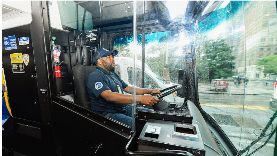
Figure 4: Bus Operator Safety Barrier with full enclosure
