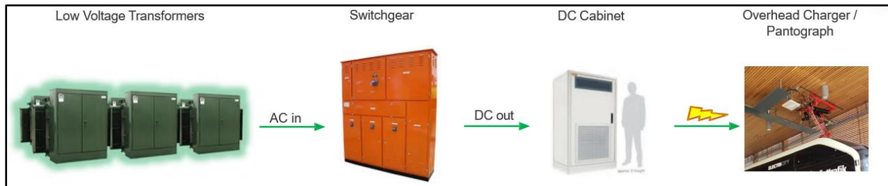
Figure 1: Battery-Electric Charging Infrastructure Overview
