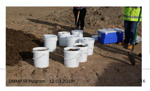
Embankment Study: Explored the use of dredged material as potential highway embankment material. This study was conducted by amending the dredged material with quarry byproducts. Geotechnical analysis was coupled with an environmental assessment to ensure satisfactory performance of the dredged material in structural fills.
