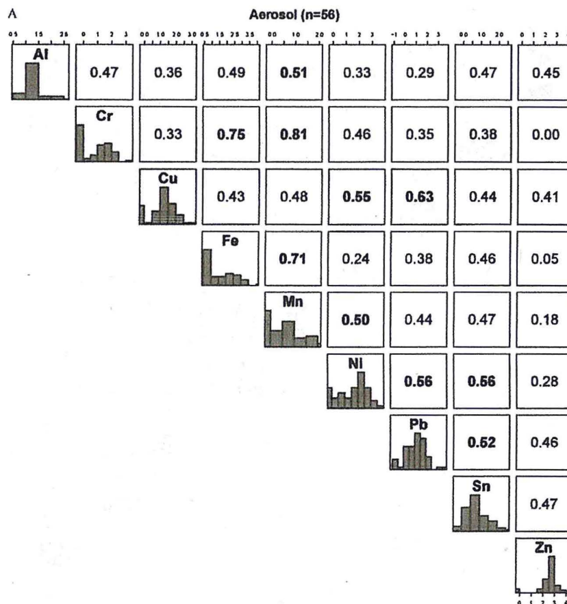
Figure 2. Correlations between metals in samples from e-cigarette devices: (A) aerosol samples, and (B) tank samples. All metals shown in Figure 1 are shown here. The diagonal panel shows the histograms of the \log_{10} -transformed distribution of each metal. The upper part of the panel represents the Spearman pairwise correlation coefficients between metals. The axes indicate the \log_{10} metal concentrations values that are represented in the histograms. Correlations \geq 0.50 are bolded.
