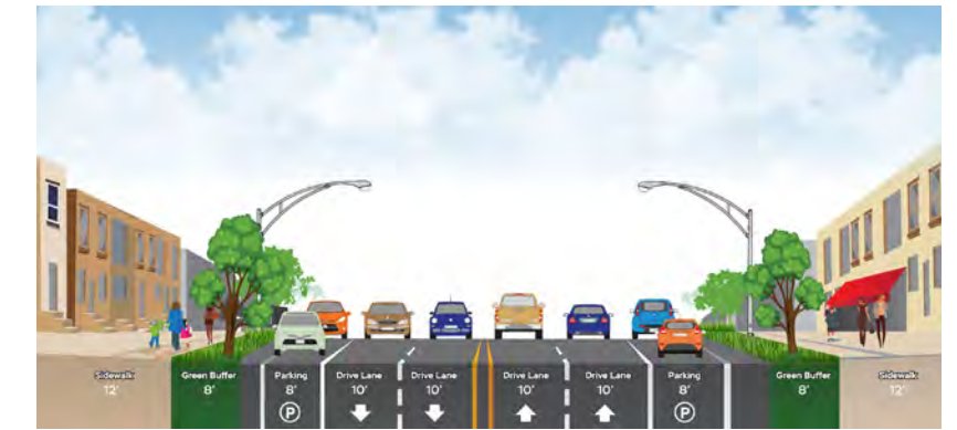
Figure 56 Typical configuration west of Bloomingdale Road
